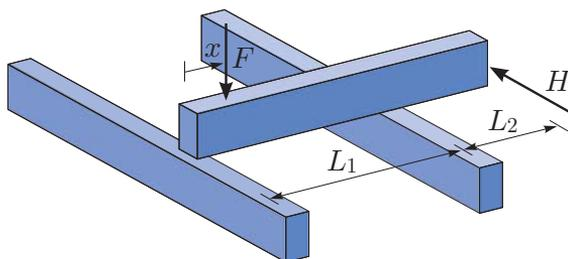
$L_1 = 6 \text{ m}$ ,  $L_2 = 3 \text{ m}$ ,  $F = 10 \text{ kN}$ ,  $k_t = 0.3$ .
