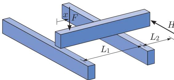
$$L_1 = 6 \text{ m}, L_2 = 3 \text{ m}, F = 10 \text{ kN}, k_l = 0.3.$$
